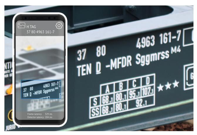
In order to reduce manual input processes in logistics management, ZEDAS GmbH has developed an AI-based wagon number recognition for RUs in freight transport.
